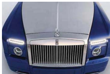
Image 6. AISI304 motor cap treated with Polinox Protect after four years of use. Photo Poligrat.
