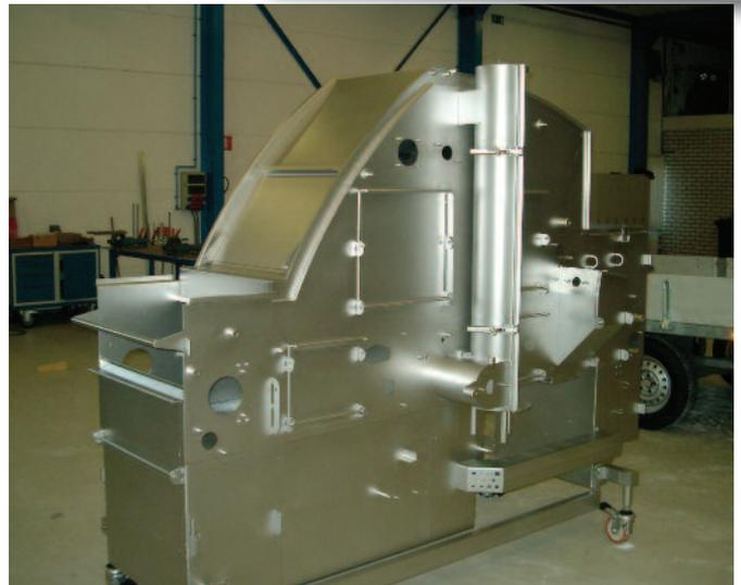
Figure 9: A breadcrumbs device treated with water blasting.
