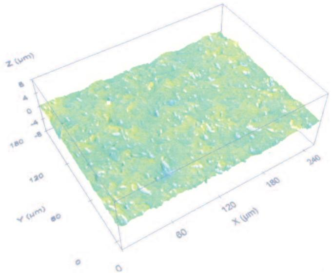
Fig. 15. Topographical 3D picture (TNO) of a water jet blasted surface with a roughness of  $0.26 \mu\text{m}$ .
