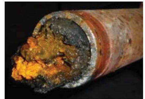
*Figure 3: Steel pipe totally clogged by corrosion products (photo: MIC Europe private company)*
