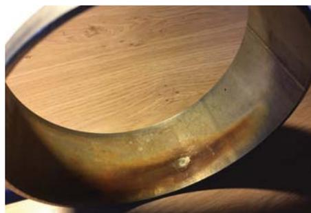
Figure 4: View of the inside of the MIC pierced 6" S10s size 316Ti pipe which had been filled with IJ river water. (photo: Innomet private company)
