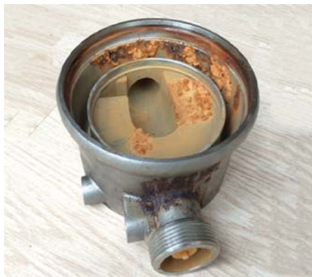
Figure 1: The foot of a pump constructed in stainless steel AISI 304 affected by MIC (photo: Innomet private company)
