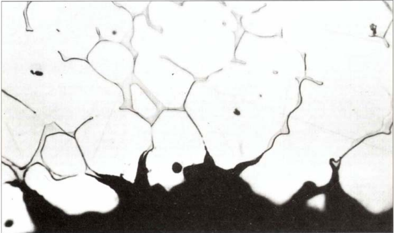
21. Preferential attack of ferrite
