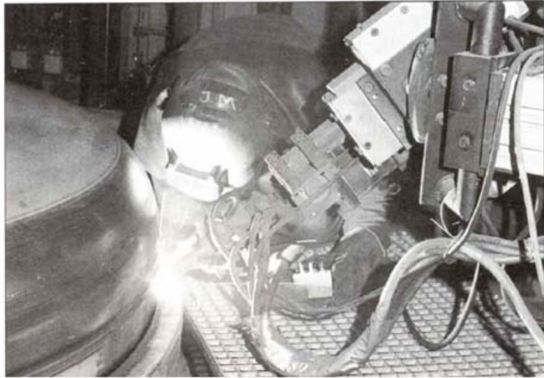
GMAW weld of a stainless steel cover
