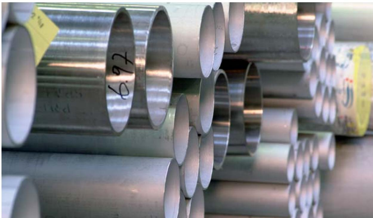
Duplex qualities are magnetic, but do not become hard. Because of the large chromium percentage and the presence of molybdenum the alloy has an excellent durability against all forms of corrosion such as stress corrosion cracking.
