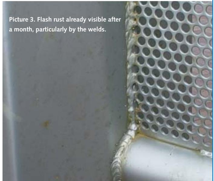
Picture 3. Flash rust already visible after a month, particularly by the welds.
