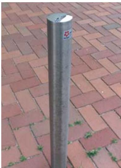
**Picture 1.** A stainless steel AISI 316 post, where all but the polished cap is corroded.
