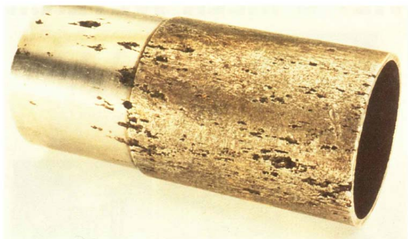
Pitcorrosion of stainless (17% Cr)
