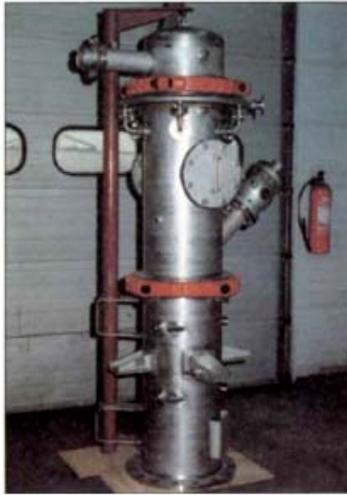
2. Filterhouse made of 316L
