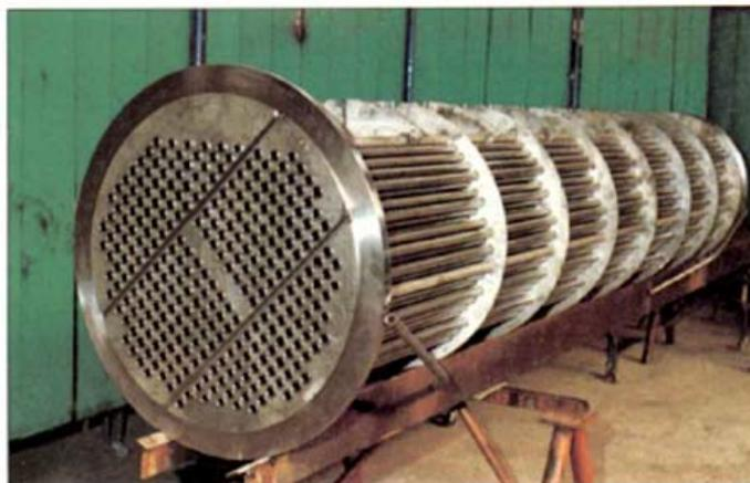
3. Heat exchanger made of 304L
