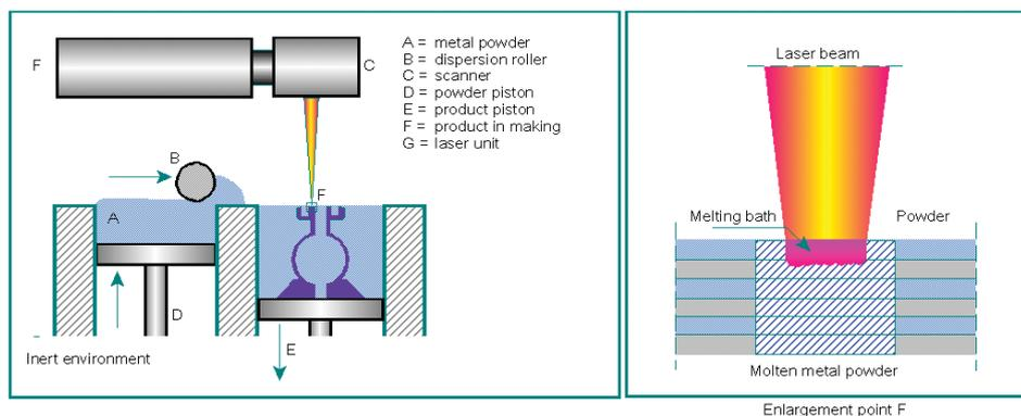
Figure 1: Schematic representation of Additive Manufacturing
