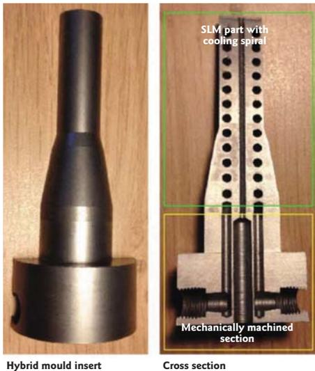
Figure 2: a hybrid product that is constructed from a mechanically worked part and a SLM part
